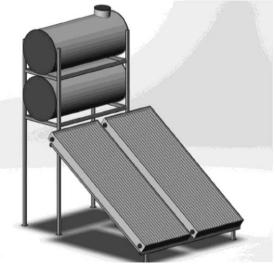
Fig. 1. Flat glazed solar collector
